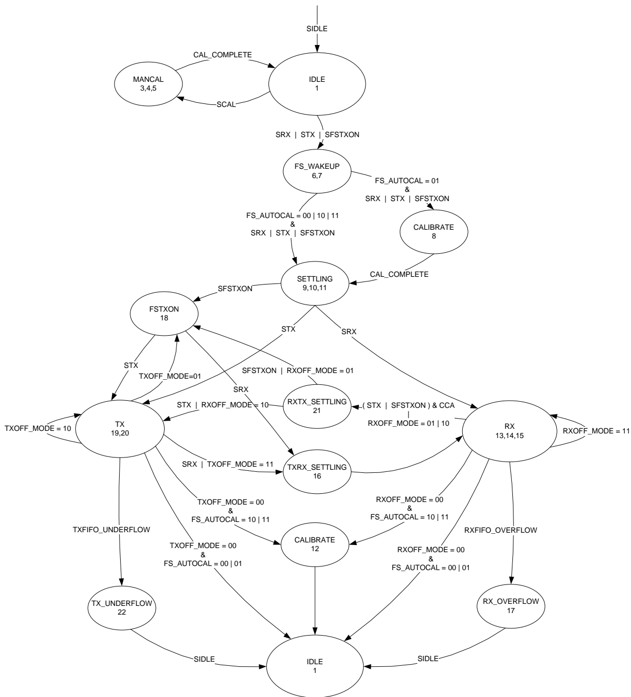
Figure 54: Complete Radio Control State Diagram
